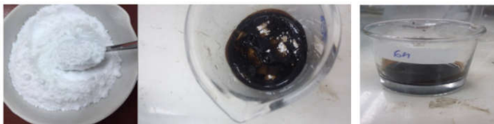
Figure 9. Experimental observation of crude oil adsorption by nanosilica LGP (sample M 20 )
